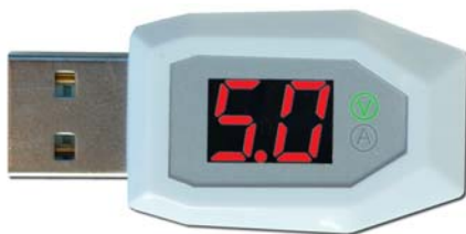
Showing voltage (when device not connected) or battery is full
